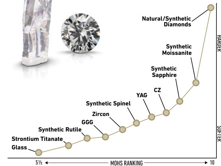
The Mohs scale measures relative gem hardness. This graph shows the hardness of natural/synthetic diamonds compared to common diamond simulants.
